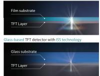
Film-based TFT detector with ISS techn
