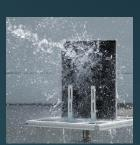
Structured to prevent the infiltration of liquids, FDR D-EVO III conforms to IPX6 standards and can withstand jets from any direction\*. There is no need to worry about fluid penetration from cleaning or body fluids. FDR D-EVO III also complies with IP5X for dust-proof protection, preventing infiltration of small
